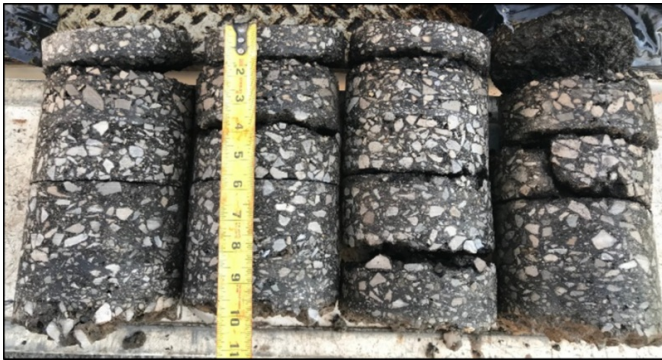
Pavement Samples taken during Investigative Sampling
