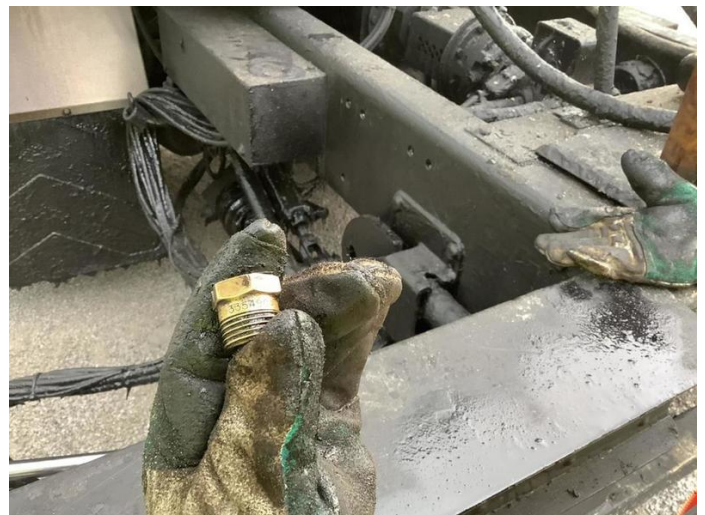
Correct Nozzle Size #3354904 which is a #1 nozzle
