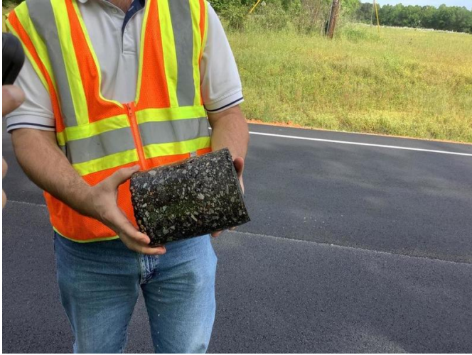
Core Cut showing tack bonded Pavement Layers
