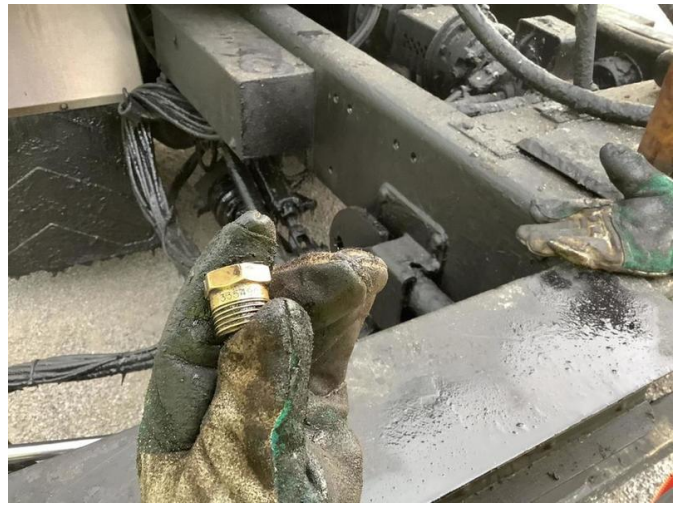
Correct Nozzle Size #3354904 which is a #1 nozzle
