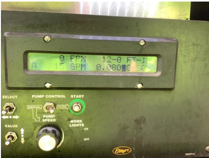
Shot Rate on Distributor Computer 0.08gal/sy
